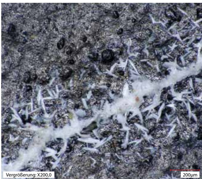
»11 Detail of a roof tile surface with efflorescences, shown after depth sharpening correction
